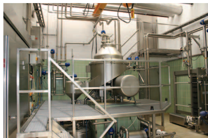
Separator for the production of curd
